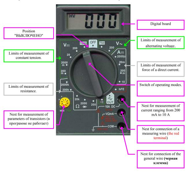
Connecting wires of the device on the screen are not shown not to encumber the bench. It is necessary for connection of the device to the studied scheme:
