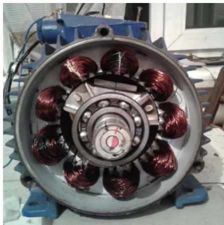
Figure 3 Photo – Symmetrically wound 9 stator windings
