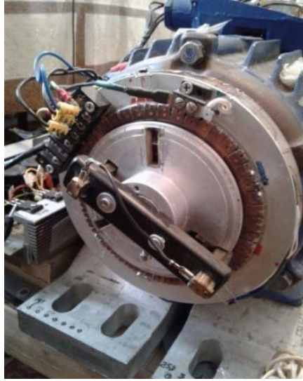
Figure 5 – Photo of manifold with contactors
