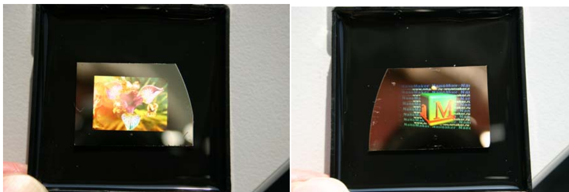
Fig. 4 – Photos showing two examples of “rainbow holograms” resulting from diffraction effects in nanoscaled grating structures which are produced in a thin resist layer using e-beam lithography. At a certain angle a colored 3D image (right) and a flower (left) are visible
